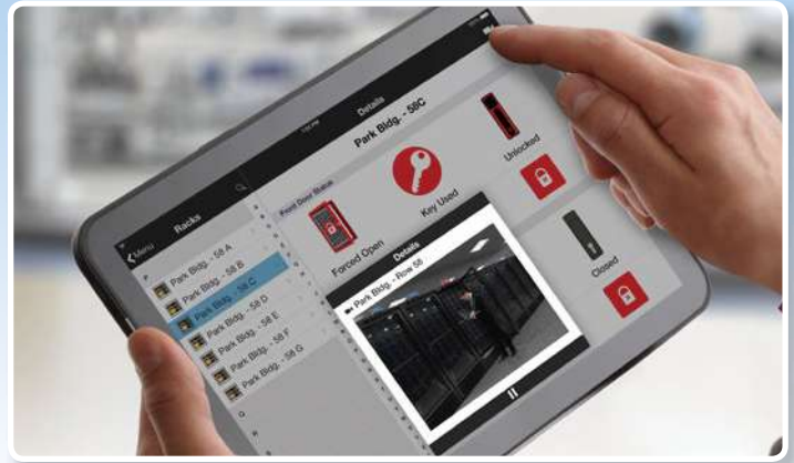
Easy graphic interface shows front/back door status of server racks per door
