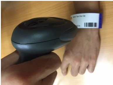
Reading of barcode printed on the wrist band using a hand held reader/scanner
